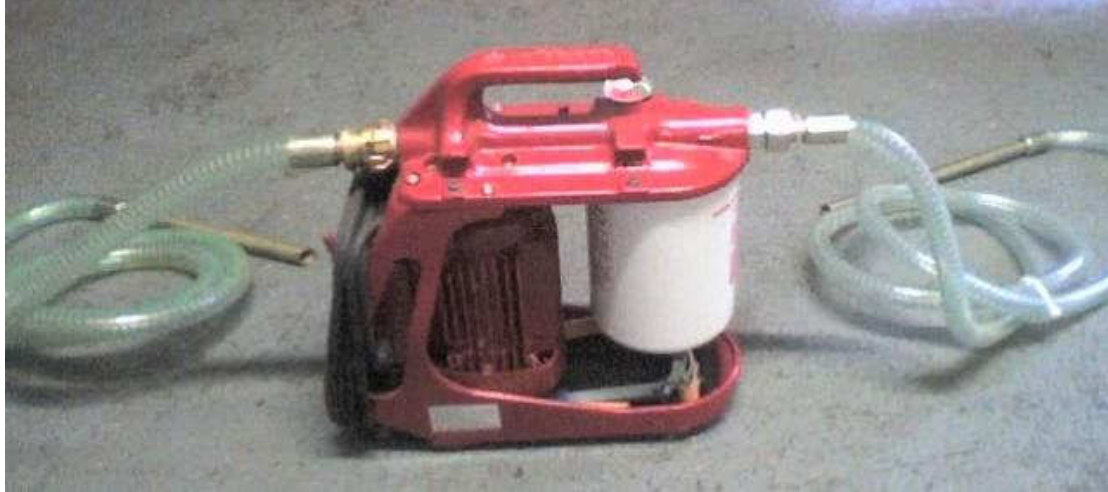
Above: OF7 portable filtration unit.
