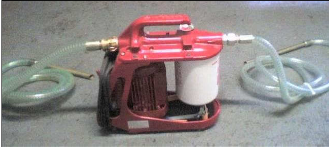
Above: OF7 portable filtration unit.
