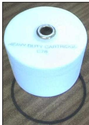
Bypass oil filtration takes a portion of the oil (around 10%) from every complete circuit cycle, through a loop system, and filters it to a fine level. In theory over many cycles the entire system oil goes through the bypass. This allows fine, gradual filtration of oil without increasing the pressure in the line. By pass filters also remove water from the oil helping to prevent engine wear and corrosion. This allows the primary oil filter to work normally and will significantly extend its life.
